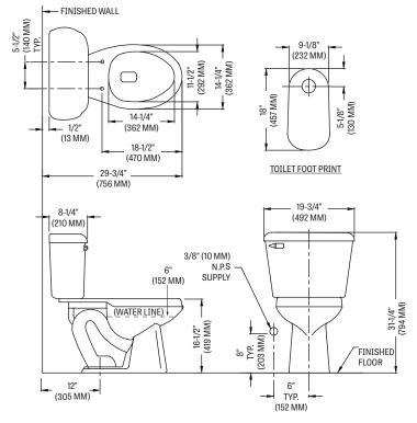
Fixture performance and specifications meet or exceed ASME A112.19.2/CSA B45.1 standards, and other state and local codes.
